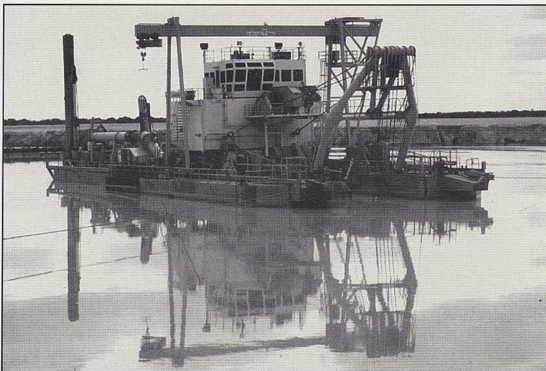
Δ A dredge for heavy mineral sands scoops the ore from a flooded basin and then despatches it to a separation plant.
