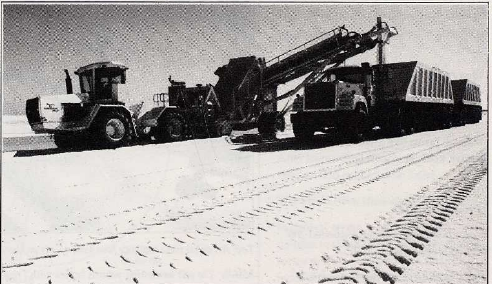
Δ Salt being harvested at Port Hedland. After the "crop" is gathered it is then taken to a wash plant.
